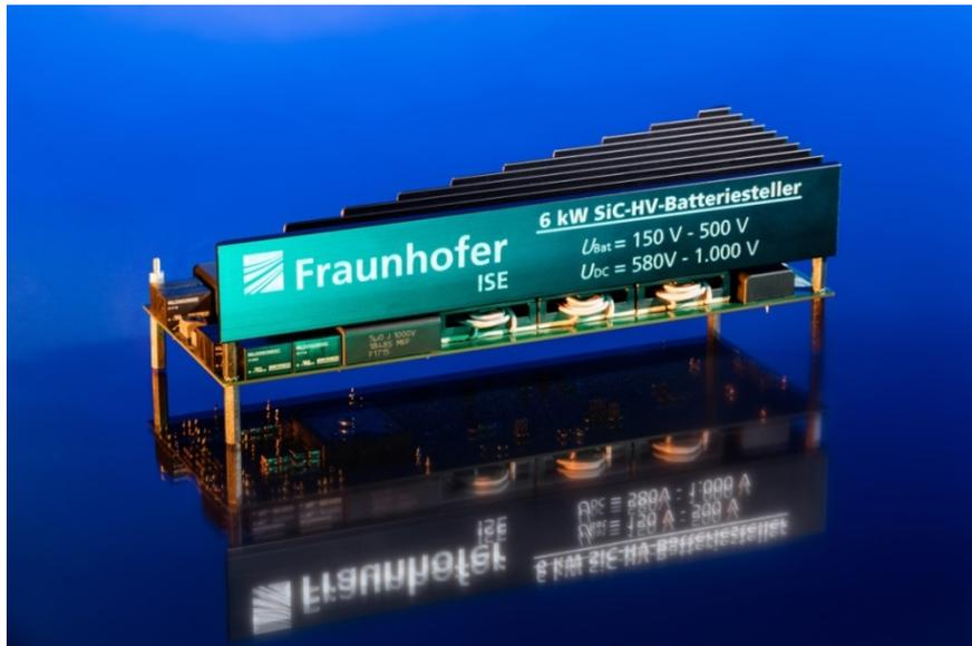
Optimized battery charger for high voltage battery with 6 kWp nominal power © Fraunhofer ISE
