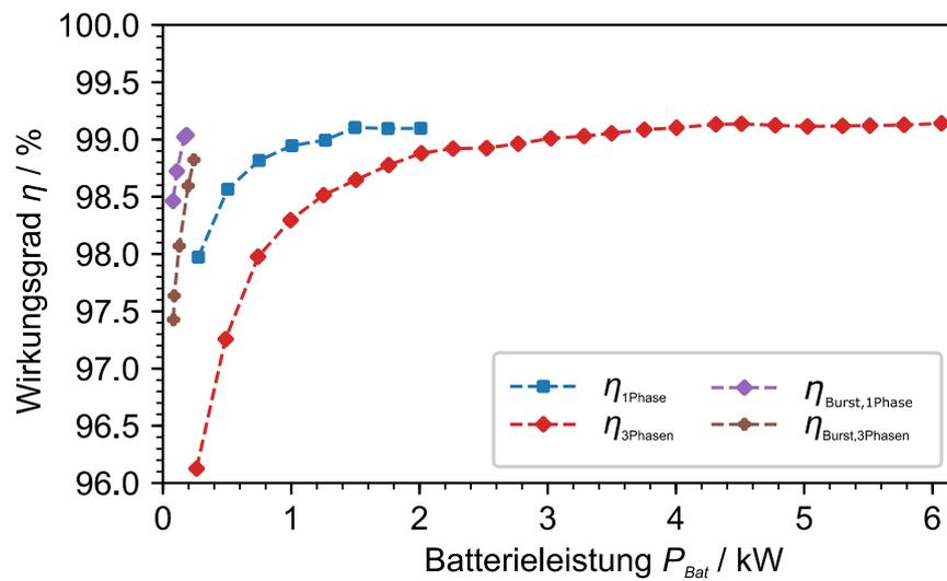
Efficiency characteristic of optimized battery charger for various operating modes: 1 or 3-phase burst operation (violet and brown), 1 or 3-phase operation (blue and red) ©Fraunhofer ISE
